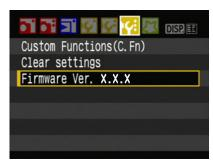
Press the Cross keys to select the "Firmware Ver.x.x.x" item at the bottom of the "Set-up 3 (Yellow)", and then press the <SET> button.
